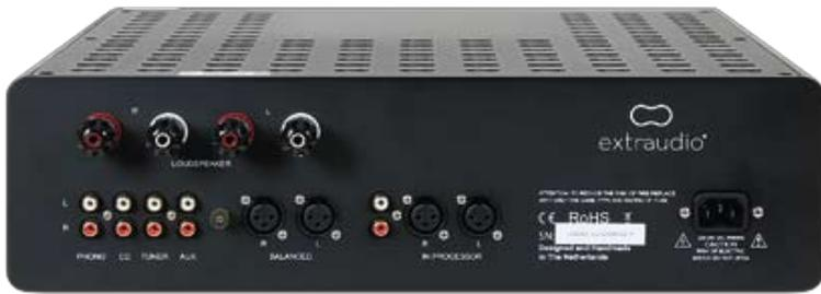
**ABOVE:** This is an 'analogue-only' amplifier with five line ins (four on RCAs and one balanced on XLRs), one of which has a MM phono option. Single-ended (RCA) and balanced (XLR) 'processor' ins connect directly to the Ncore power amp. The 4mm speaker cable outlets use high quality WBT connectors
